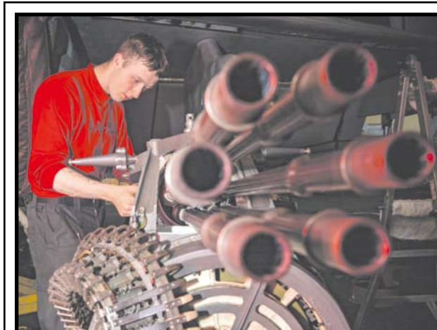
SOUTH CHINA SEA (Feb. 13, 2023) - Navy Aviation Ordnanceman Airman Patrick Tripp inspects an M61A2 20 mm gun aboard aircraft carrier Nimitz. US Navy photo by MC3 Caylen McCutcheon
