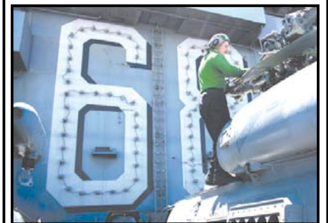
PHILIPPINE SEA (March 10, 2023) Aviation Structural Mechanic 3rd Class Austin Whitehead services the main rotor head on an MH-60R Sea Hawk helicopter on the flight deck of aircraft carrier Nimitz. US Navy photo by MC3 Joseph Calabrese
