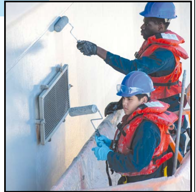
ABOARD USS TRIPOLI (May 3, 2023) Seaman Wilson Alumonah, from Lagos, Nigeria, right, and Seaman Edgar Rosales, from San Marcus, Texas, paint the hull of amphibious assault ship Tripoli during the ship's maintenance availability. Tripoli is an America-class amphibious assault ship homeported in San Diego. US Navy photo by MC1 Danian C. Douglas
