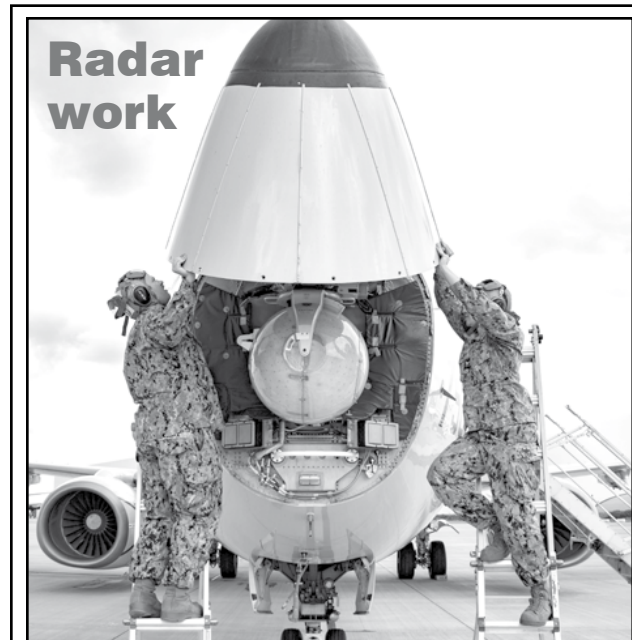
ROYAL AIR FORCE LOSSIEMOUTH, U.K. (July 15, 2023) Aviation Electronics Technician 2nd Class Colton Berka, left, and Aviation Electronics Technician 2nd Class Diego Olvera, assigned to the Golden Swordsmen of Patrol Squadron (VP) 47, perform maintenance on the AN/APY-10 radar of a P-8A Poseidon here. VP-47 is currently deployed to the 6th Fleet in support of naval operations to maintain maritime stability and security in order to ensure access, deter aggression and defend U.S., allied and partner interests. U.S. Navy photo by MC1 William Sykes
