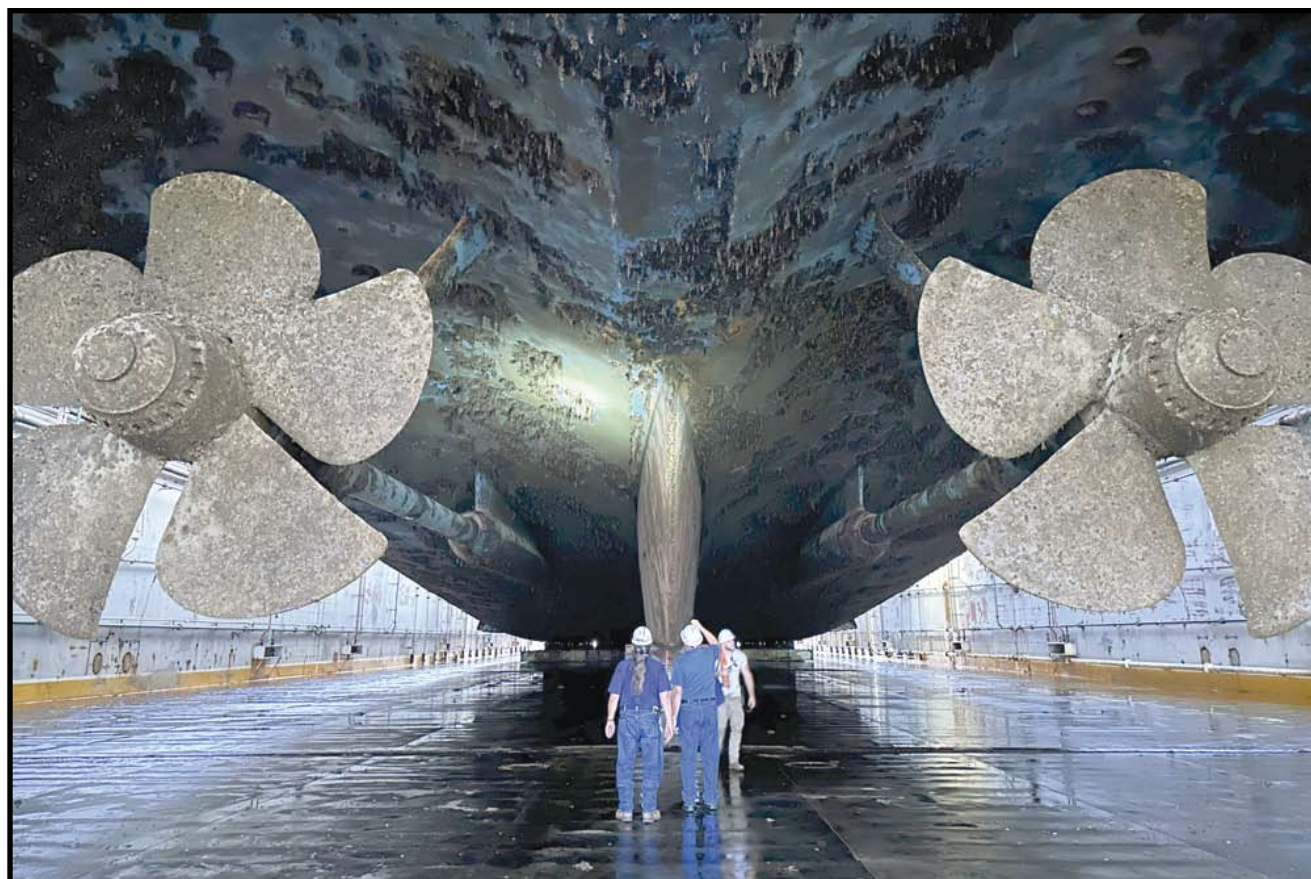
Keel Check - Shipyard personnel examine USS Arlington's keel at a dry dock in Norfolk, Va., recently. Arlington is undergoing scheduled maintenance and upgrades to increase warfighting capabilities and capacity. U.S. Navy photo by Lt. Cmdr. Nathaniel Bendickson
