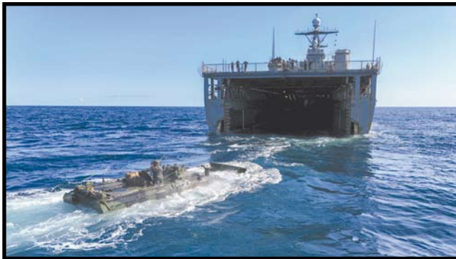
USS HARPERS FERRY, at sea (Sept. 4, 2024) An Amphibious Combat Vehicle from Battalion Landing Team (BLT) 1/5, 15th Marine Expeditionary Unit, enters the well deck of amphibious dock landing ship USS Harpers Ferry (LSD 49) during exercise Ssang Yong 24 in waters east of the coast of South Korea. Exercise SY24 strengthens the Republic of Korea-U.S. Alliance through bilateral, joint training, contributing toward combined amphibious capability in defense of the Korean Peninsula. U.S. Navy photo by MC2 Sang Kim
