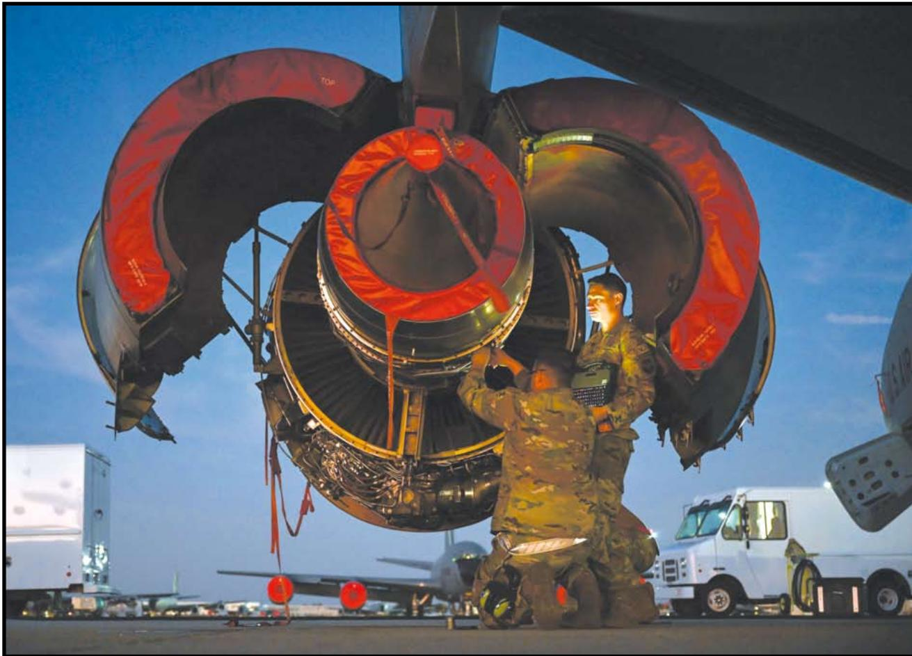
**TAKING A LOOK UNDER THE HOOD** Aerospace propulsion Airmen assigned to the 6th Maintenance Squadron inspect the engine of a KC-135 Stratotanker at MacDill Air Force Base, Fla., earlier this month. Aerospace propulsion specialists are responsible for the maintenance, repair and testing of aircraft engines, turbines and other propulsion systems. U.S. Air Force photo by Senior Airman Derrick Bole
